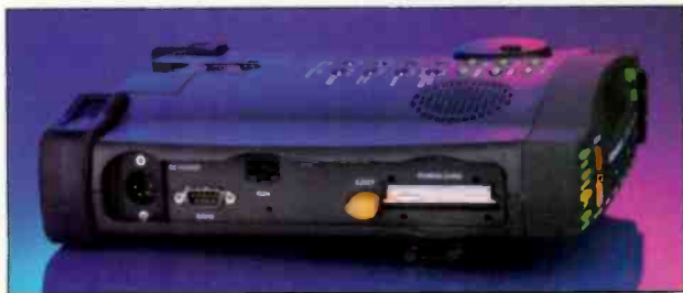
The side panel has power, serial data and ISDN jacks. The PC card slot accepts Type II or Type III cards.
