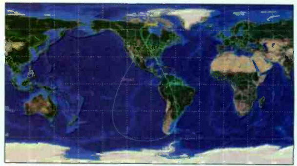
Figure 2. The effective Sirius satellite coverage factoring the orbital paths and Earth's rotation.
