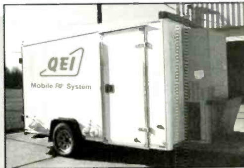
Transportable Pre-Built Transmitter Sites
