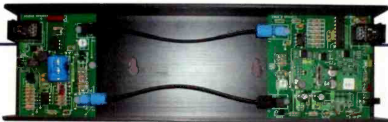
Inside view of the unit showing the fiber optic protection connection.
