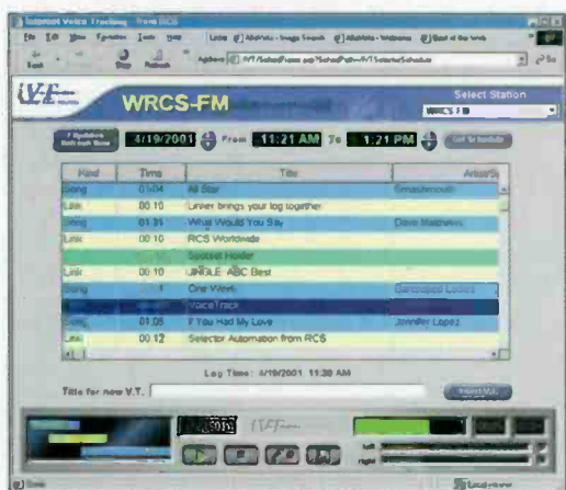
Voice tracking, in-studio or via the Internet, is a widely used function of automation systems.
