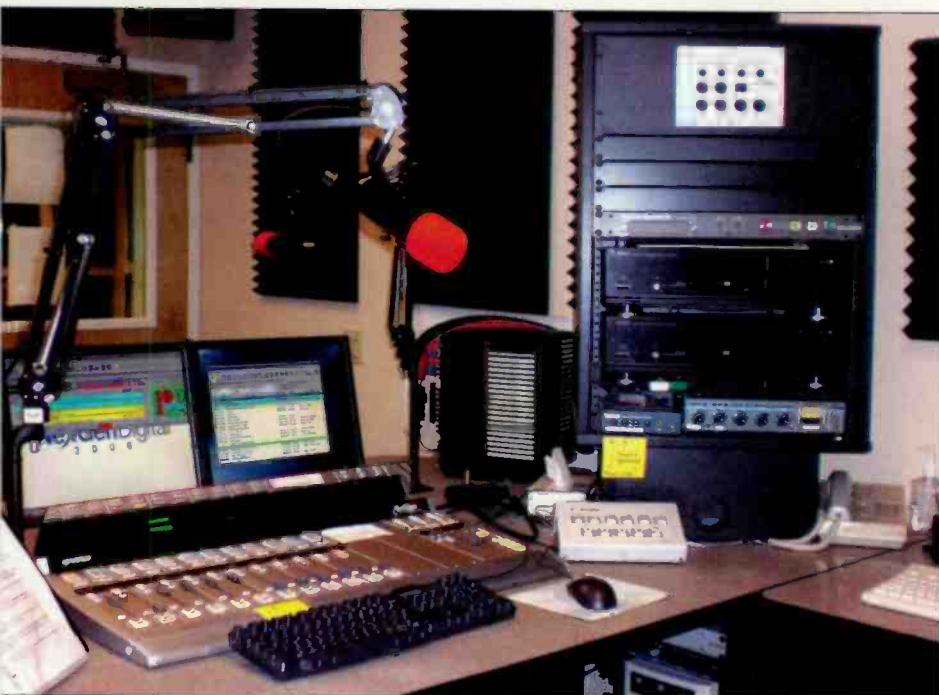
The KODS-FM studio is centered around a Harris Netwave console and Prophet Nexgen automation. Rack equipment at KODS includes Denon CD players and a Gentner Digital Hybrid II phone system. A Harris World Feed panel for plug-in systems is integrated into the top of this rack.
