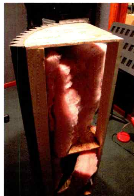
The completed trap showing before installation
