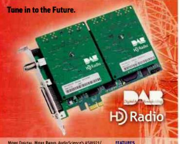
MORE DIGITAL. MORE RADIO. AudioScience's ASI8921/ 8821-5500 series tuner cards offer the most digital radio capabilites: 4 or 8 tuners for analog FM, HD-Radio FM or DAB/DAB+. Record streams in PCM, MPEG-1 layer2 and MP3, while capturing all associated PAD data.
