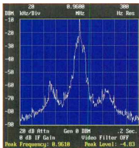
Figure 3. Spurs due to AM TX power supply
