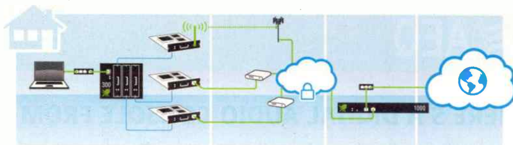
The data stream from the LAN is encrypted by the Multichannel VPN Router and distributed onto the Internet connections (here 2x DSL, 1x 3G / UMTS). The encrypted and fragmented data passes the networks of the utilized ISPs and reaches the Multichannel VPN Hub in the data center, which in turn decrypts the data stream and reassembles it correctly. Afterwards, the data stream is forwarded to its actual destination on the Internet. The same goes for the opposite direction. Here, the Hub encrypts the data stream, while the VPN Router decrypts it.
