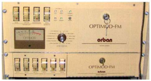
Figure 1: Orban Optimod 8100-FM with XT chassis
