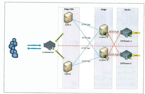
Fig. 1: Network configuration for RTL's streaming service (flows right to left)
