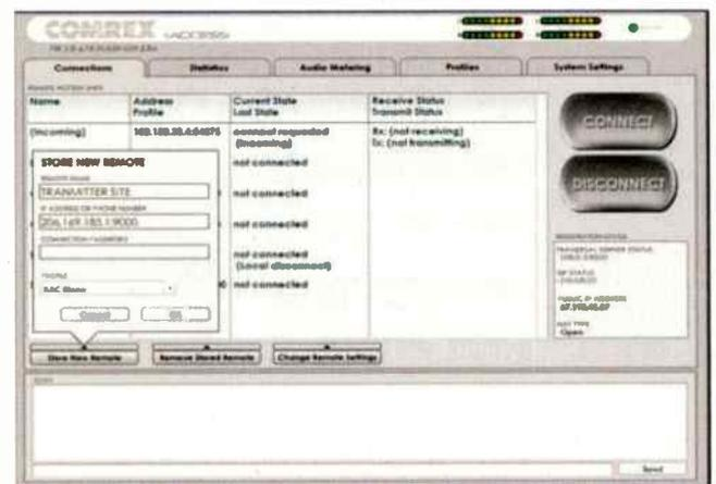
Fig. 3: Configuring a new remote connection
