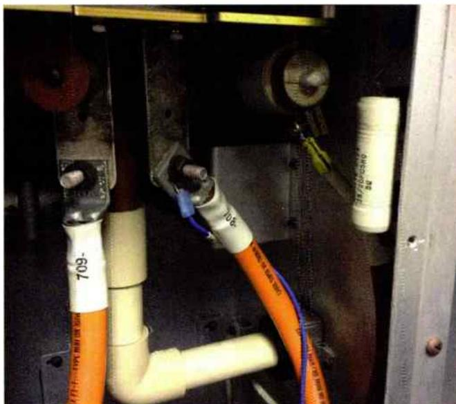
The final amplifier input section (below the tube socket) should be clean and inspected for loose or broken parts as part of the rebuild process.
