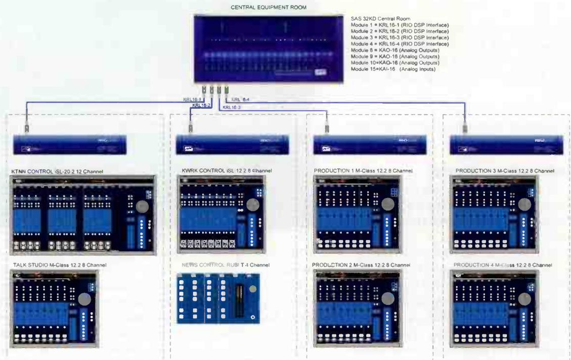
SAS system design for the KTNN facility, showing locations of i-SL, Rubi-T and M-Class control surfaces.
