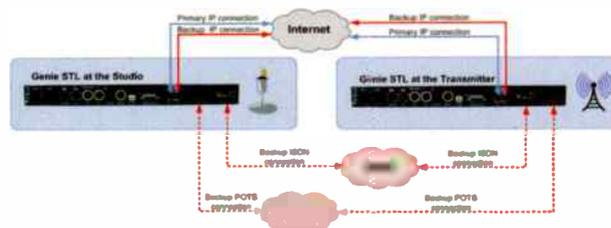
In addition to two IP network connections, the end-user can configure the Tieline Genie STL to make use of ISDN or POTS for end-to-end connectivity.
