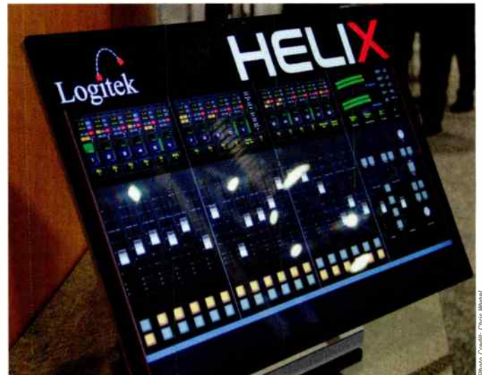
The Logitek Helix is but one example of the virtualized control surface.
