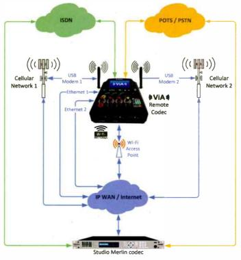
Tieline's Fuse-IP data aggregation technology enables the user to bond multiple IP interfaces for a more reliable connection.
