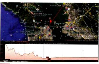
From the top: Add a placemark for your site; after selecting a second point of reference, measure the elevation; and save the elevation profile.
