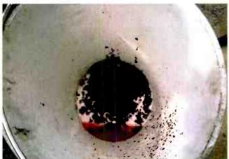
Fig. 4: This particulate matter was removed from 300-gallon diesel tank.
