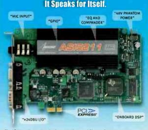
The ASI5211. Not another dumb card. With a microphone input, including a low noise pre-amp and 48V phantom power supply, on-board DSP, increased analog I/O level of +24dBu and a new GPIO that adds two opto-isolated inputs and two normally open relay outputs, the ASI5211 is one smart card. And considering it's priced the same as cards without all these features, it's one smart choice, too. For information, call +1-302-324-5333 or email salesasi@audioscience.com. ASI 5211 features:
