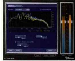
else. RX 2 Advanced extends the standard RX with an adaptive denoiser mode, a deconstruct module, third party plug-in hosting, iZotope 64-bit SRC resampling, MBIT+ dither, iZotope Radius time and pitch control, ability to export an edit history, multi-resclution mode for Spectral Repair and automatic azimuth correction. New visual editing features are also featured.
