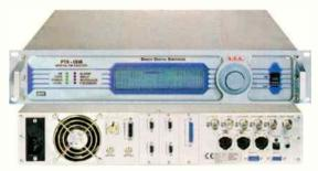
**PTX100-DDS:** PTX100-DDS uses DSP technology complying with all EC, FCC and CCiR standards. It features a built-in digital stereo coder, ITU professional limiter and on-board RDS, and AES/EBU, L/R, mono and MPX inputs, auxiliary inputs for SCA/RDS signals. It is completely microprocessor controlled, easy to program via menu or RS-232, and all main parameters are displayed on the LCD screen. It interfaces with all RVR telemetry systems to guarantee simple remote control of operating parameters.
