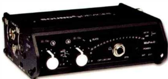
cameras and devices used in production today, it has output adaptability and serves as an flexible, class-compliant USB audio interface. The MixPre-D offers numerous analog output options including mic/line switchable balanced XLR, dedicated consumer mic-level on a locking TA3 connector and an aux-level output on 3.5mm connection. Digital outputs include balanced AES3 on XLR and USB audio connectivity.
