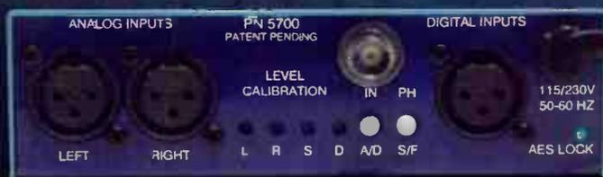
The **Stereo Audio Monitor (SAM)** is a stereo level and phase meter that incorporates Single Stereo Display\* technology. SAM provides a visual indication of the levels and phase relationships of a stereo audio signal. The unit indicates the usual Left and Right channel levels, and also displays the Sum and Difference components of the stereo signal.
