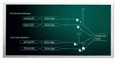
Figure 3. Separate transmitter configurations
