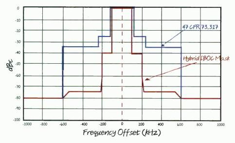
Figure 5. Comparison of FM hybrid mask and FCC mask
