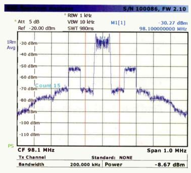
Figure 8. Combined IBOC and modulated analog signal with undesired energy.
