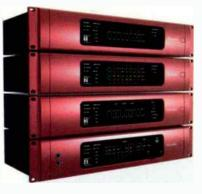
RedNet: At this professional audio networking system's heart is digital audio networking technology Dante by Audinate. Dante uses conventional IP-based Ethernet switches to carry up to 256 channels (128 inputs and 128 outputs) of high-resolution digital audio over a single, standard Ethernet network. RedNet provides extremely low latency: under 3ms analog-to-analog at any sample
