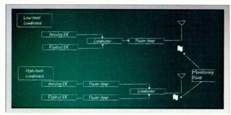
Figure 2. Combined transmitter configurations
