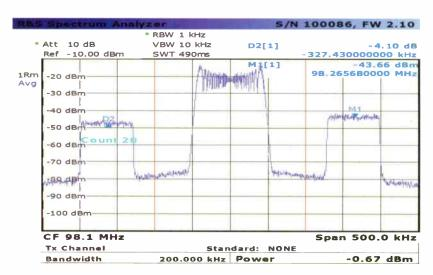
Figure 9. Asymmetric FM hybrid spectrum
