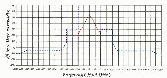
Figure 4. FM IBOC transmission mask
