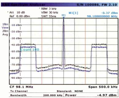
Figure 1. FM hybrid IBOC signal without modulation
