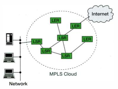
Figure 1. An MPLS cloud has data enter through an Ingress Edge Router (LER), travel through the Label Switch Router (LSR) and then back to an Egress Edge Router to its next destination.
