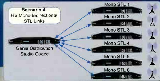
Connect 3 independent stereo streams or, 2 stereo + 2 mono, or 1 stereo + 4 mono, or 6 mono streams
