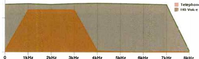
To qualify as HD Voice, the codec used must sample the voice at a minimum of 16kHz, at least doubling the audio bandwidth available. In addition to adding in high frequencies, HD Voice restores the low end (below 300Hz) that gets filtered by most phone networks. The result is a crisper, more intelligible conversation with a
