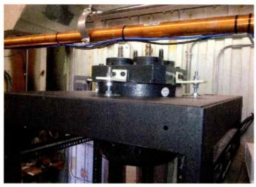
Figure 3: Four-Port Switch Mounted in the Top of the Equipment Rack
