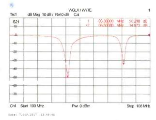
Network analyzer characterization of notch-filters to be used ahead of spectrum analyzer input. These filters reduce the amount of the fundamental signals getting in to the analyzer, which effectively increases the dynamic range of the measurement, allowing an easier "capture" of the actual
