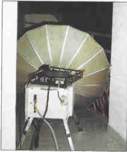
Rear view of MAGNAPhone shows codec (black box) connecting to transmit/receive unit via V.35 cable. The black cable at center feeds audio from mixer to codec. The gray cable snaking off to the right connects the control console to the transceiver.
