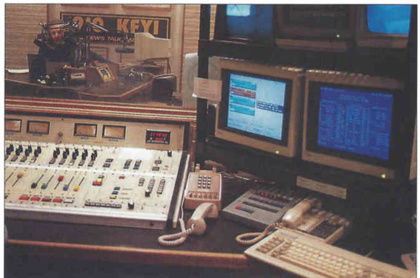
Call screening station in control room at KFYZ, Phoenix. Light blue graphics screen (left monitor on lower shelf) shows caller data. This display also appears on host's monitor in studio.
