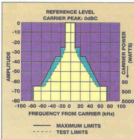
Figure 1. The NRSC-2 emission standard's RF mask. Note differences in last step for different stations' licensed power levels.
