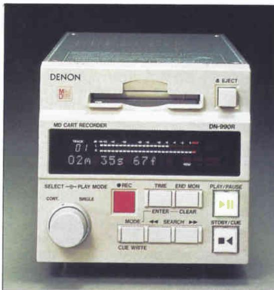
The Denon DN-990R is an example of new digital cart machine recorders using the MiniDisc format.
