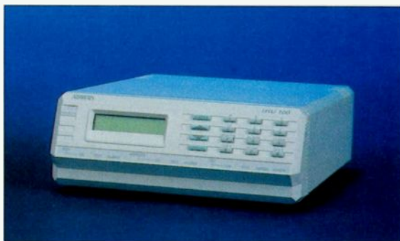
The Adtran HSU-100 is an example of currently available ADSL modems.
