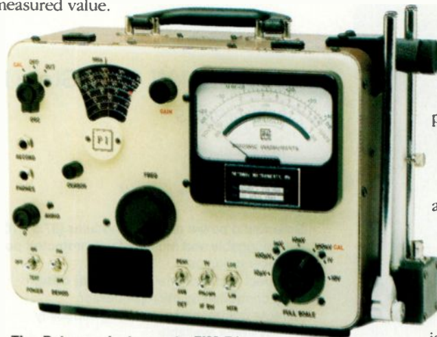
The Potomac Instruments FIM-71 field intensity meter — a familiar sight at FM proofs.
