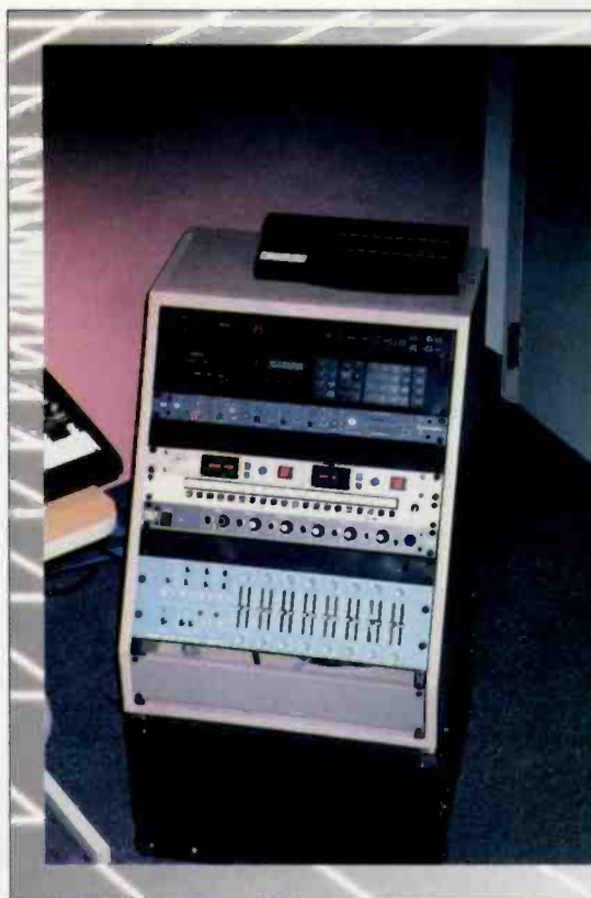
Outboard equipment should be placed where it accessible to the operator. Equipment that is accessed more frequently is at the top.
