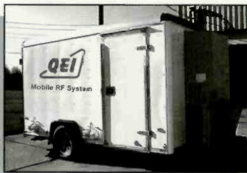
Transportable Pre-Built Transmitter Sites
