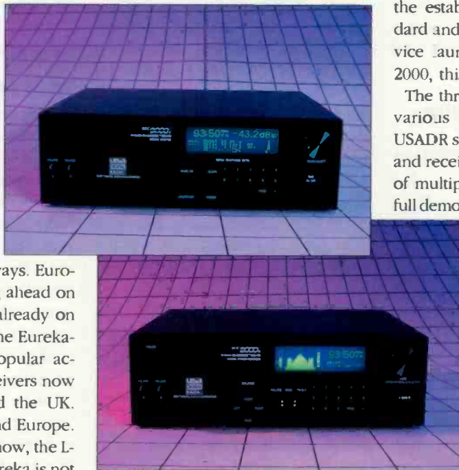
Test prototype IBOC exciter (top) and receiver that were shown by USADR at the NAB Radio Show.
