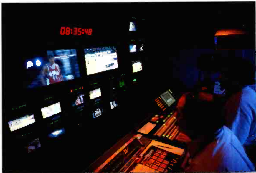
All picture monitoring in HDV-5 is full HD quality, allowing the director and TD to evaluate the framing, composition and overall image quality without making allowances for the shortcomings of LCD flat-panels or NTSC downconversion. Photo courtesy WRAL-TV.
