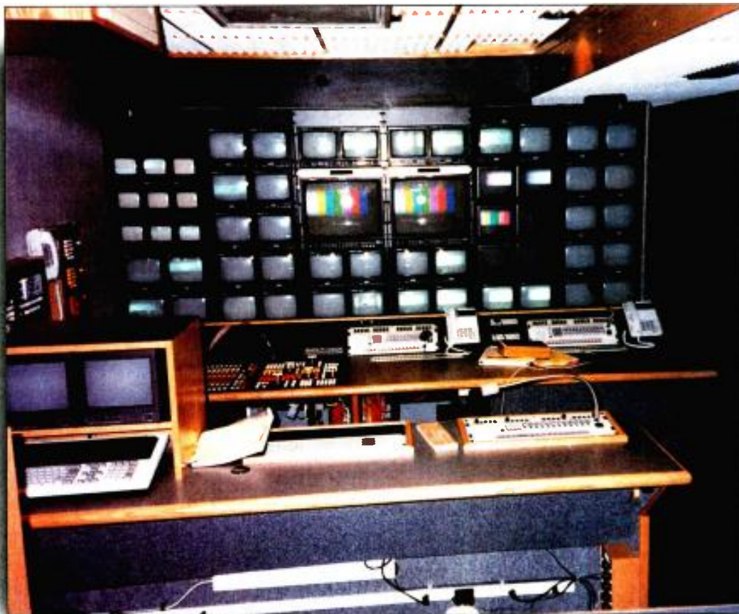
Before beginning an upgrade, carefully consider the floorplan for the vehicle's trailer. In an expando unit, production monitor sightlines must be carefully considered.
