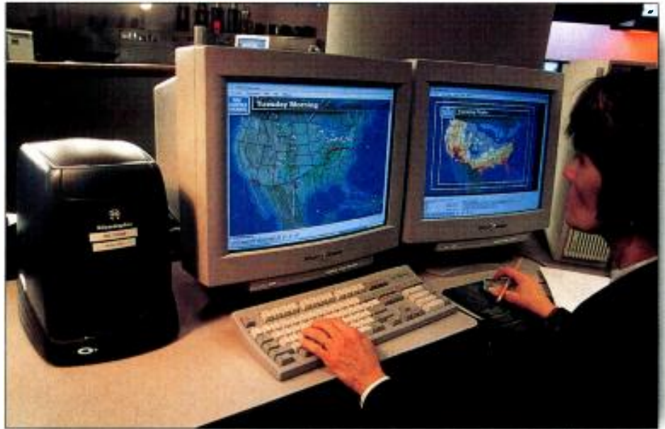
The Weather Channel's forecasting system includes two SGI Origin 2000s, 35 SGI O2 and seven SGI Octane workstations running Weather Services International's WxPro software. Photo by Tim Olive, courtesy of SGI.
