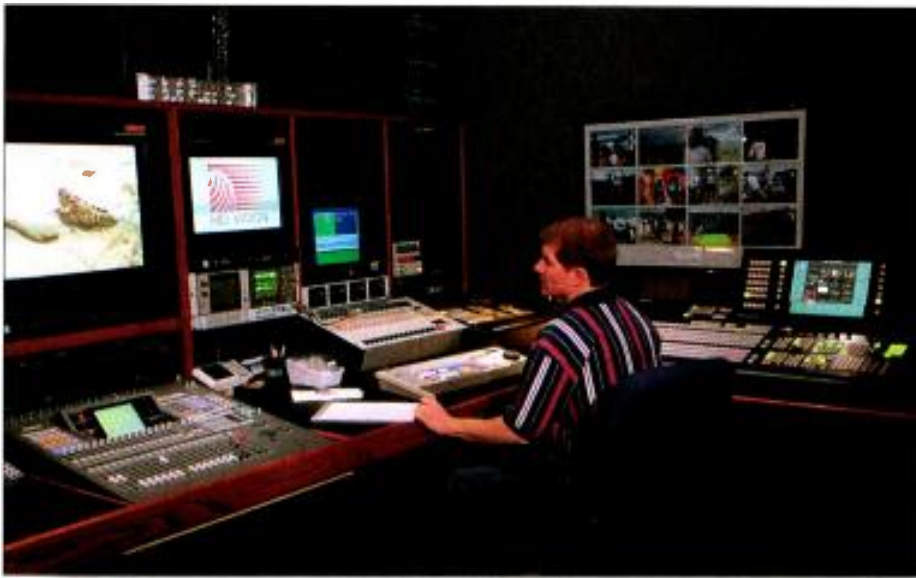
The linear HD suite is connected to Sony HDD 1000s, Panasonic D-5 HDs, Sony HDCAMS, and even a Sony UNI-HI for recording and playback.
