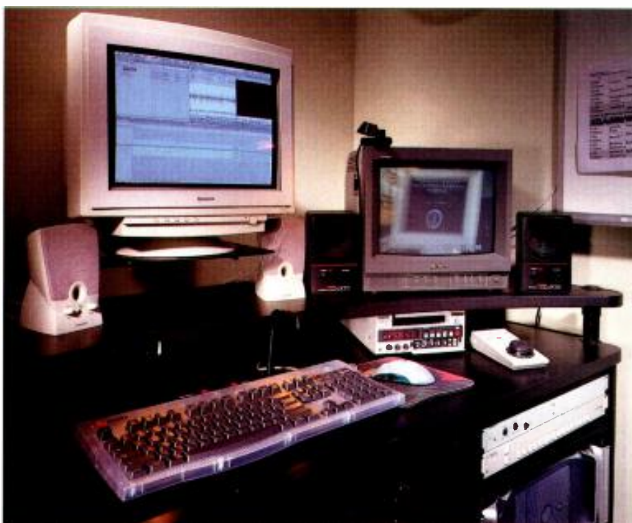
Desktop edit stations utilize Apple Final Cut Pro and Sony DVCAM tape machines with IEEE 1394 digital I/O technology.
