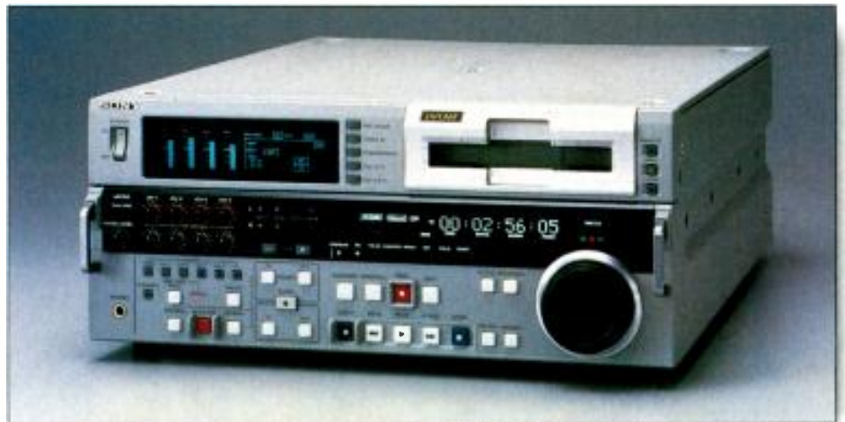
The Sony DSR-2000 DVCAM digital video recorder/player is useful in television stations and professional video production companies for its DVCAM format, which allows for component digital video recording using a 1/4-inch cassette tape and the ability to play back other DV format tapes.
