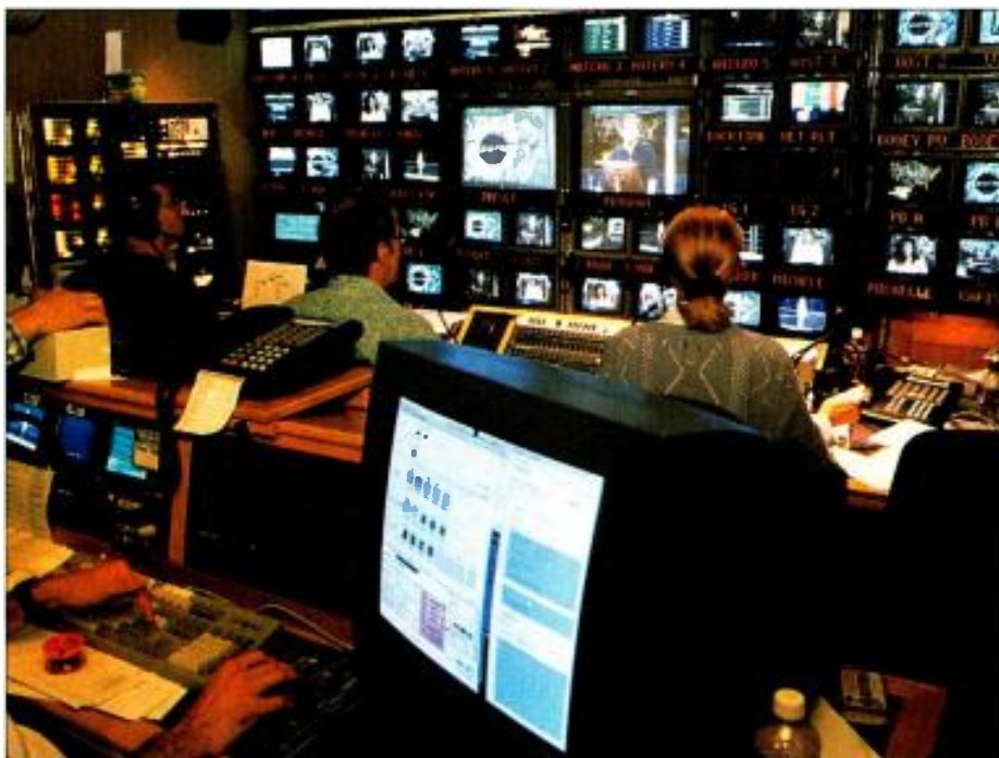
Remote satellite and Internet contestants are graphically fed into Paranoia live using RT-SET's Antero software running on six SGI Octane visual workstations.
