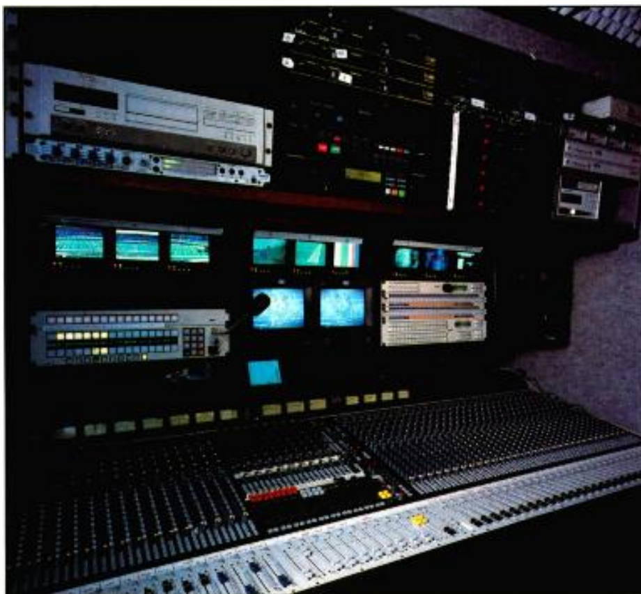
In building an audio mixing system for use in remote operations, extra channels for potential on-air requirements of a live production such as off-camera announcer mics and VTR insertion playback should be included in order to save upgrading later.
