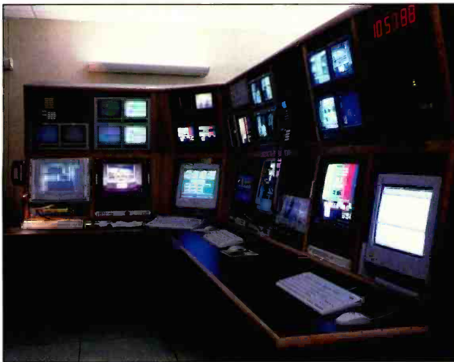
ENG microwave, satellite receive and analog to digital QC in KPDX's facility is accomplished at multiple quality control monitoring points, or "QC stations." The station shown above is compact, allowing ease of control over multiple sources.
