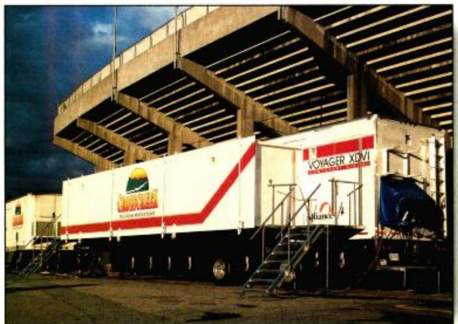
Remote trucks feature an expanding street-side wall. Space for audio operations is often limited in an effort to conserve space in remote trucks, but inadequate human space can be detrimental to show quality.
