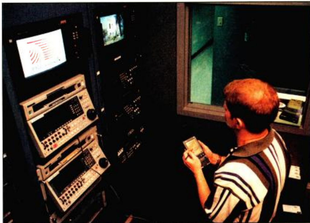
Pocket Producer's intuitive display functions like an edit controller, with in and out mark points, a duration indicator, and standard play, pause, stop, rewind, and shuttle controls. The device also offers Tag functions that allow operators to choose the reference point for the clip.
