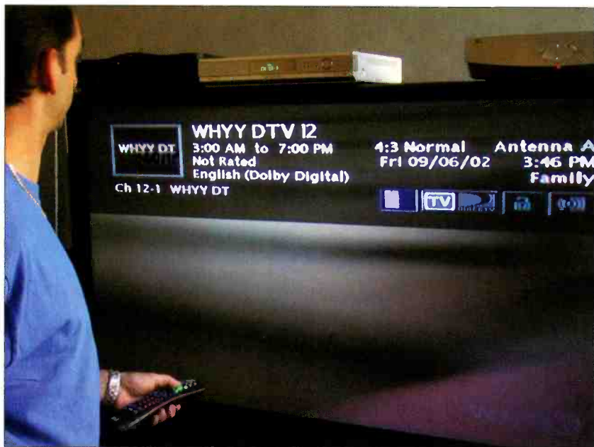
This photo shows the two-part channel number and other on-screen information made possible by PSIP. Photo courtesy Triveni Digital.
