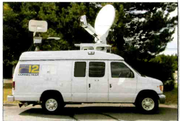
The Wolf Coach ENG/SNG van offers hybrid terrestrial RF transmit and digital Ku uplink capabilities in a smaller-profile unit.
