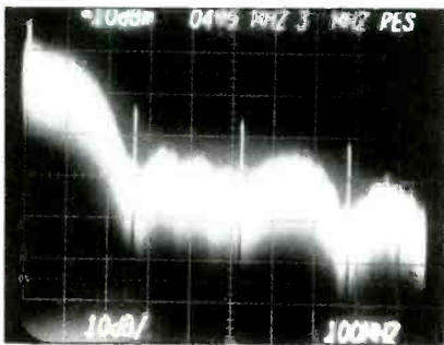
Figure 2. Spectrum of 270Mb/s 4:2:2 component digital bit-serial signal
