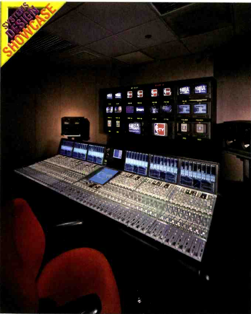
The centerpiece of NBAE's new networked audio suite is Solid State Logic's C100 digital broadcast audio console. It is configured with 96 channels and 48 faders, and can handle both a stereo and live 5.1 Dolby Digital AC-3 mix from the same interface.
