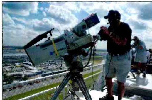
Sony's HDC-910 can capture 1080i 50/60 images and output them as 1080i 50/60, 480i 60 or 720p 60.
