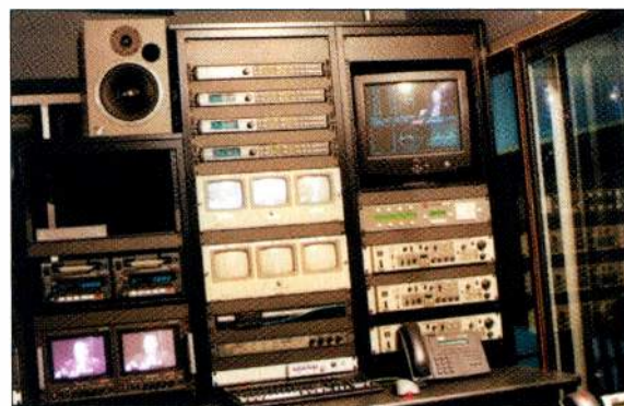
The production studio engineer position controls the video levels, encoders and client copy tape decks.
