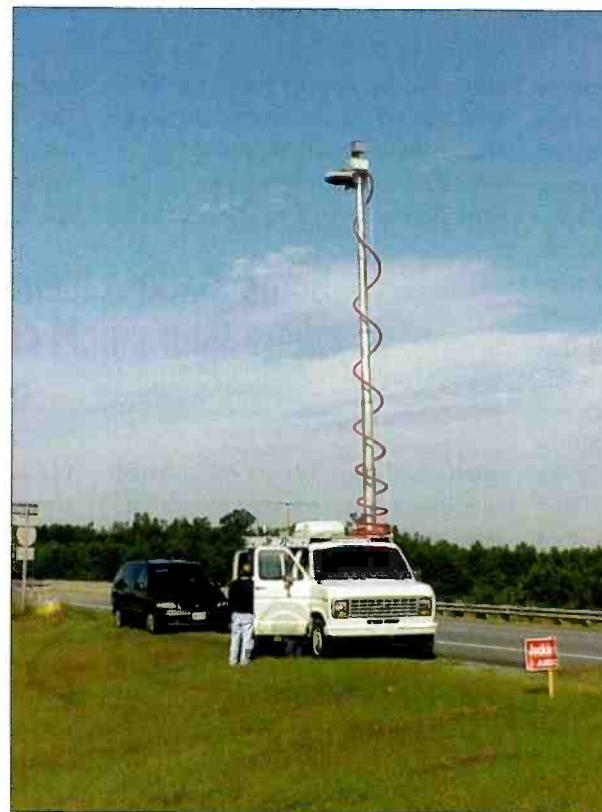
Stations sometimes must conduct field-strength measurements to verify coverage. This truck is operated by WRAL-TV, NC. Photo courtesy Potomac Instruments.
