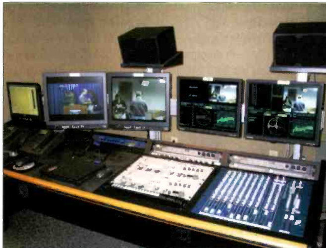
The production control area of the Center for Disease Control’s HD press room in Atlanta is equipped with all-HD equipment including Evertz’s conversion and signal processing systems, and Panasonic’s AK-HC900 720p cameras and AJ-HD1700 archive video recorder. Photo courtesy Digital Systems Technology.
