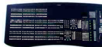
2 M/E Control Panel
