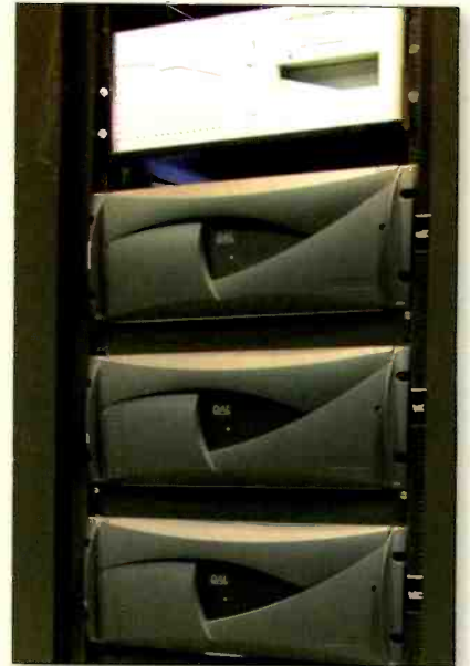
The broadcaster uses Harris automation computers (shown above). Content that is redistributed to regional local transmitters across the country contains local regional branding, logos and crawls, which are inserted from branding systems in Montreal.
