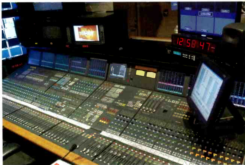
A Calrec Sigma digital audio console (with Bluefin DSP technology) is used in the network's new 2K audio control room, which feeds taped segments to "The Today Show's" Studio 1A.
