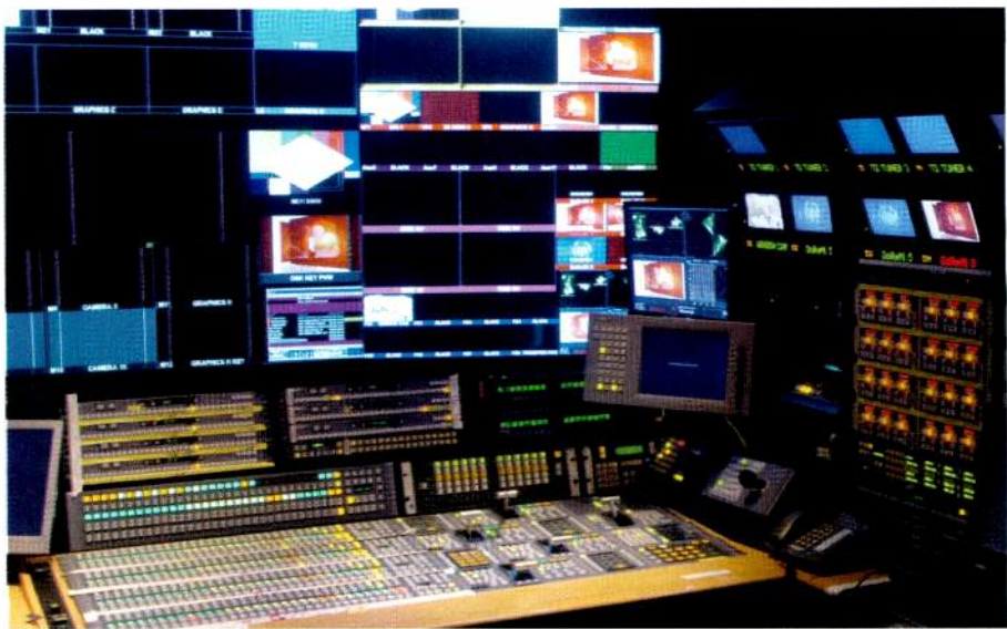
The main control room's Sony MVS-8000 HD production switcher is used for a variety of multilayered effects during the live show and also for pretaped segments.
