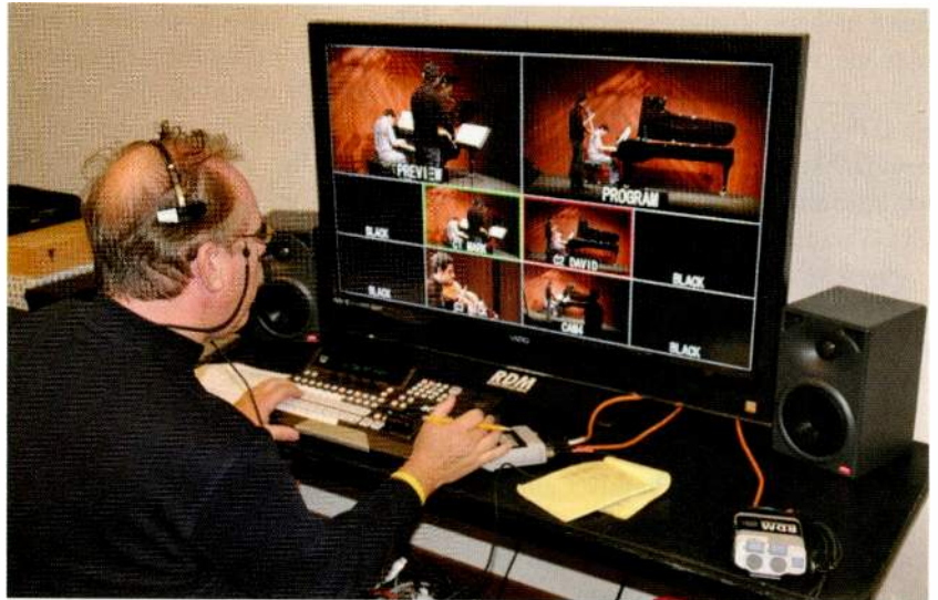
Sandor Bondorowsky, an owner of Remote Digital Media in Montclair, NJ, uses a FOR-A HVS-300 switcher during the production of a concert at the Nokia Theater Times Square in New York City. The HD unit supports 1080i, 720p and SD sources.
