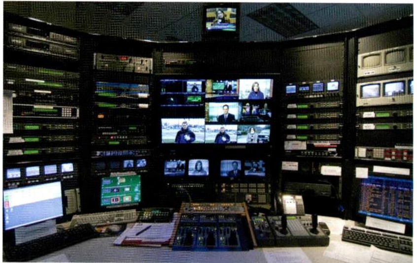
Lexington, KY, NBC affiliate WLEX-TV recently converted its automated master control system to HD, which included the installation of a Harris IconMaster switcher and IconStation advanced channel branding station.
