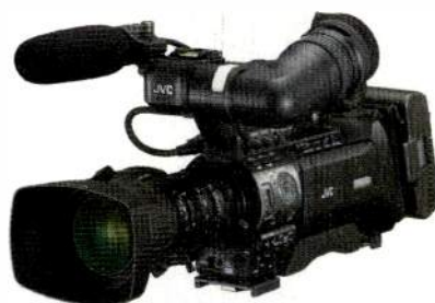
The GY-HM700 weighs 8lbs and uses three 1/3in progressive scan 1280 x 720 CCDs. Both the HM700 and HM100 record two channels of uncompressed 16-bit audio at 48kHz when recording at 25Mb/s and 35Mb/s.
