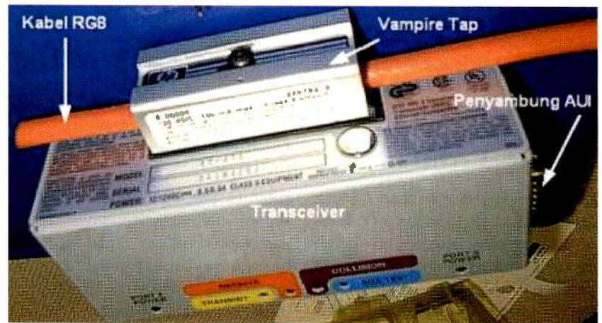
Figure 1. Illustrated here is a vampire tap transceiver showing the medium access unit and a DB-15 attachment unit interface connector, which connects the tap to the computer.
