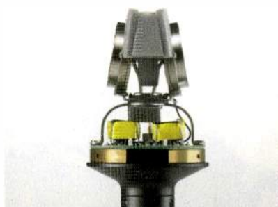
While some X-Y mics incorporate two physical capsules mounted on a handle, others, such as the one shown here, use proprietary engineering techniques to achieve an X-Y arrangement inside a more traditional headcase.
