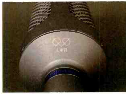
Most stereo mics are marked as to proper indication. Be sure that the proper end is up (left) in order to maintain L-R perspective (right).
