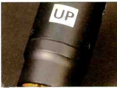
Most stereo mics are marked as to proper indication. Be sure that the proper end is up (left) in order to maintain L-R perspective (right).
