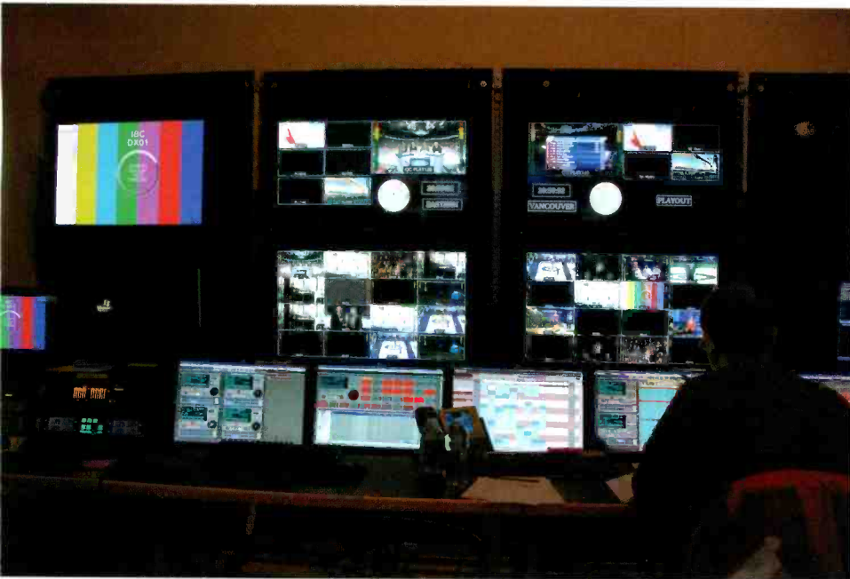
Panasonic flat-panel plasma HD displays and TVLogic monitors displaying Evertz MVP and VIP multiviewer software were strategically located throughout the CTV complex to help monitor the hundreds of feeds coming into the IBC in Vancouver.
