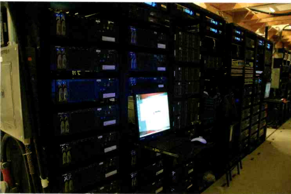
All broadcast material was recorded to a large Harris Nexio AMP server (with dual 15TB arrays and 32 ingest ports), and editors working on Harris Velocity HD edit workstations built video clips in English and French for the various program distribution platforms.
