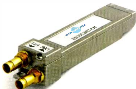
The EB30CSRT-LN SFP transceiver module is designed to transmit and receive SDI signals up to 2.97Gb/s over 75Ω coaxial cables via DIN 1.0/2.3 connectors.
