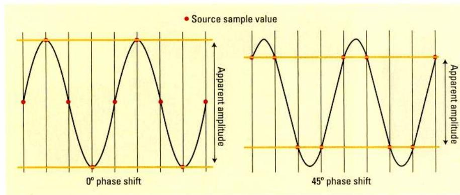
Figure 3. A peak-sample meter given the same tone as above (12,000.1Hz) will show the level dip four times every 10 seconds as the phase shifts, leading to an under-read of the level.
