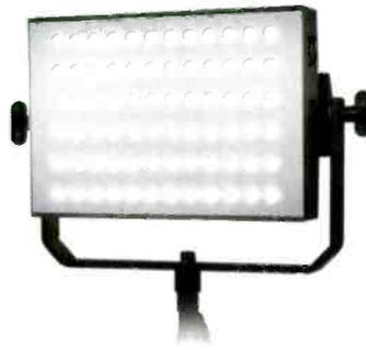
LED fixture is capable of throwing illumination over a 6.1m to 7.6m distance; is 5600°K color balanced, using an array of 72 1W daylight LEDs that are focused to a 10° angle; the 100W H2 fixtures provide light equivalent to a 1000W legacy lighting fixture, using just 10 percent of the energy; generates no noticeable heat; provides dimming from 100 percent to zero with no noticeable color change.
