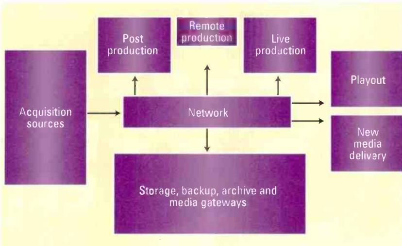
Figure 2. A high-speed network is the backbone of a content management system.
