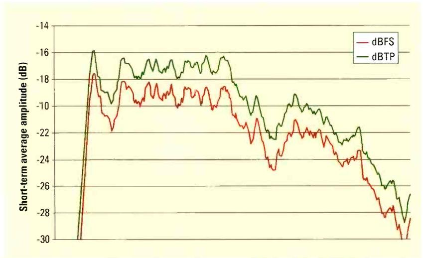
Figure 1. A comparison of the peak-sample amplitude vs. the true-peak amplitude, both averaged over a short period of time, shows that using peak-sample metering results in an average under-read of about 2dB.
