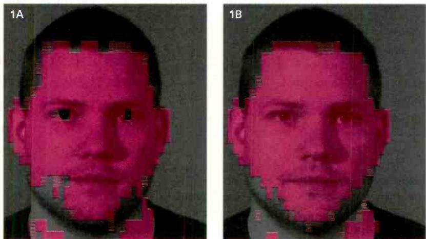
Figure 1A. Detected skin regions without applying morphology algorithms are shown in pink, and as a result, the eyes are not part of the ROI. Figure 1B. After applying morphology algorithms, the complete face is marked as ROI.
