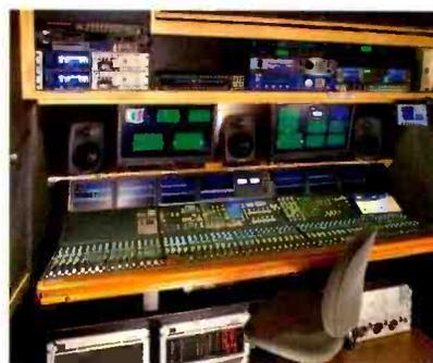
Above: The truck's production area has a full-size Evertz monitor wall, a Grass Valley production switcher at the front, and accommodations for producers and graphics staff in a second tier. Upper right: The equipment area has compact racks and router frames to conserve space. Lower right: The Calrec audio console can mix stereo and full surround sound productions.
