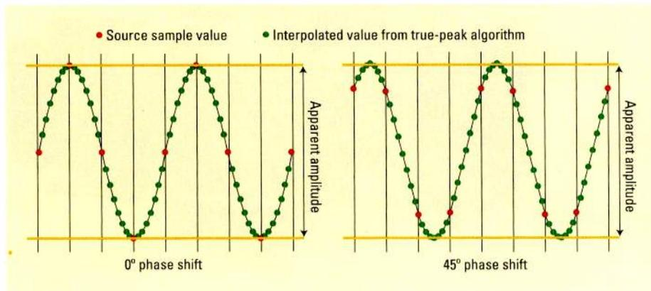
Figure 2. When given a test tone that is just off an integer division of a sample frequency (12,000.1Hz for 48kHz), a meter that uses a true-peak algorithm will show a steady level as the audio plays.
