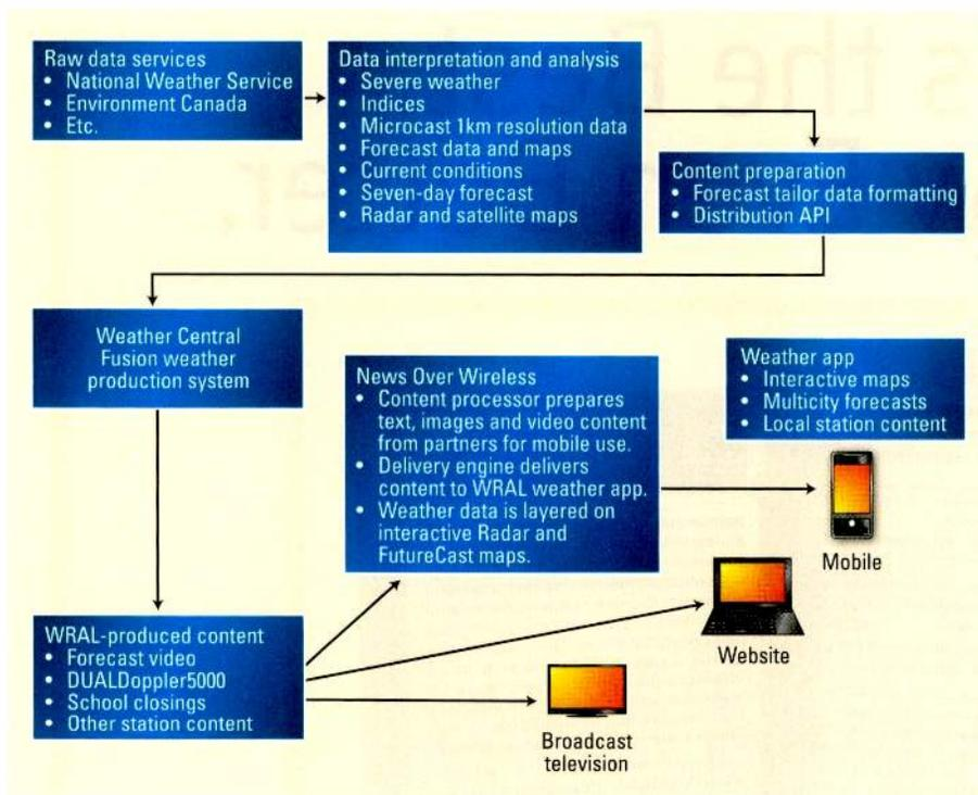
**Figure 1. The workflow for WRAL's weather application takes advantage of the station's application programming interface (API) to provide a link between the app and a comprehensive data set.**
