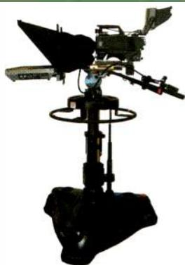
Pan-and-tilt head has a maximum payload of 83.8lbs for portable cameras with viewfinders and prompts; robust structure and wide range of balance supports a versatile variety of camera configurations; mount can be either flat base or 150mm ball.
