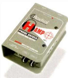
Speaker-to-headphone converter allows two sets of headphones to be driven directly from a speaker connection or amplifier output; equipped with two Neutrik Speakon fittings; speaker signal is converted to a safe mono-adjustable output for headphones; multiple H-Amps can be used in series by adding more Speakon NC4 cables.
