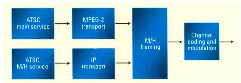
Figure 1. The ATSC mobile service works alongside the existing main service.
