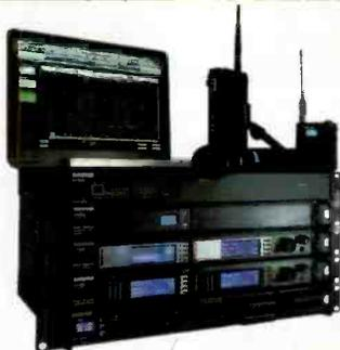
Wireless microphone system can automatically change frequencies — undetected by the user — to avoid interference; detects RF interference and moves to a clear and compatible frequency in milliseconds; has frequency diversity, which transmits full-bandwidth audio on two separate frequencies to ensure seamless, uninterrupted audio for mission-critical channels.
