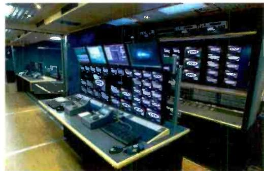
Above: The camera shading and engineering control area is dedicated to nearly a dozen Ikegami HD cameras and coordination of a number of the truck's sophisticated production systems. Right: Two six-channel EVS XT2 servers along with an EVS XFile and an IPDirector are used primarily for editorial, file record and transmission to master control.
