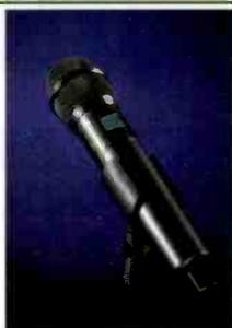
Handheld transmitter is newest addition to line of digital hybrid wireless microphone systems; accepts standard thread-on capsules from a number of manufacturers; two capsules are available from Lectrosonics, the HHC cardioids condenser and the HHS supercardioid condenser — giving users the freedom to select the microphone capsule best suited for their particular application; offers 44dB of input range; is equipped with a membrane switch control panel and high-resolution LCD display.
