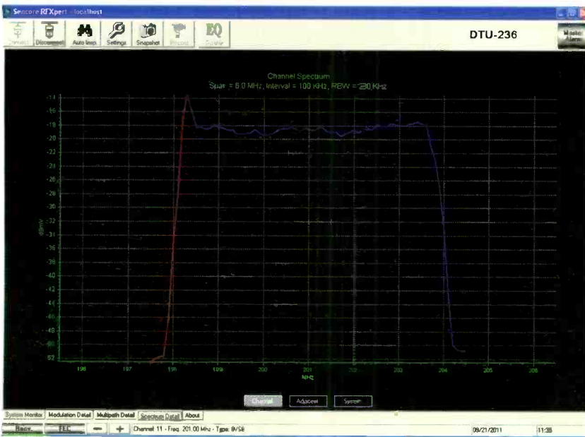
Figure 5. A spectrum analyzer shows the signal power as it is dispersed across the channel band. Variations from the ideal flatness of the signal level through the center of the band indicate frequency or phase distortions.
