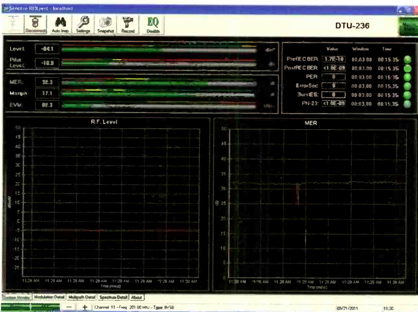
Figure 4. For MER, the larger the value, the better the signal quality. Typical performance of an 8-VSB transmitter should approach, if not exceed, a value of 30dB.
