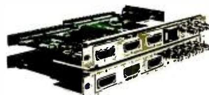
Multiviewers integrated directly into routers reduce the need for external video processors.
