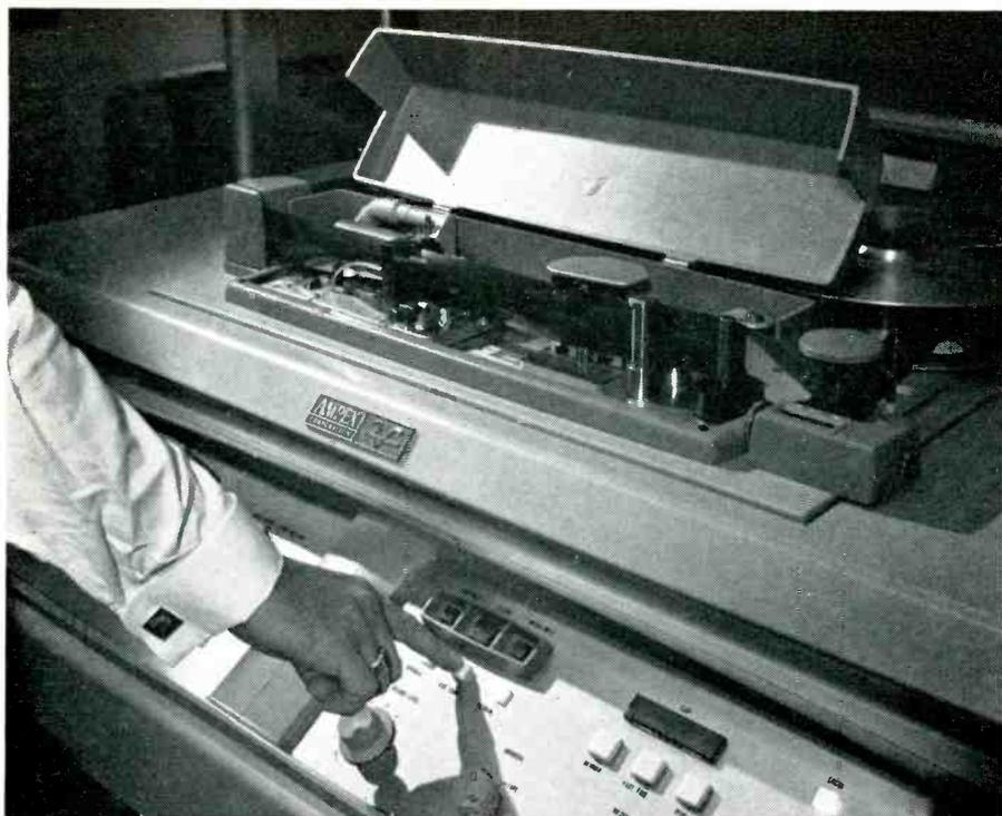
Front view of VTR console, showing tape transport system and push button controls.
