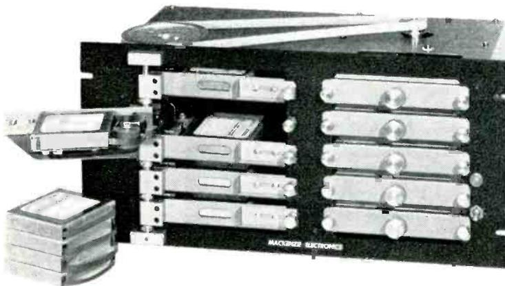
Write, wire or phone collect, for further information, specifications and delivery. The Model 5CPB shown here features five channels, each with individual plug-in transistorized pre-amplifiers and separate gain controls.
