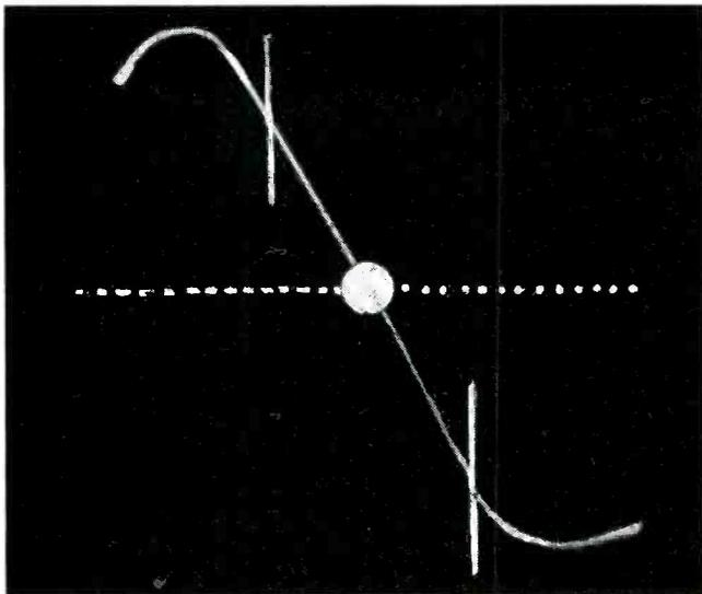
Fig. 4—In the case of a correctly adjusted receiver, the large white dot in the center of the linear portion of the "S" curve represents the position of the carrier. The two vertical lines are drawn in to show the relative positions of the upper and lower 65 Kc. sidebands when the subcarrier is being transmitted.
