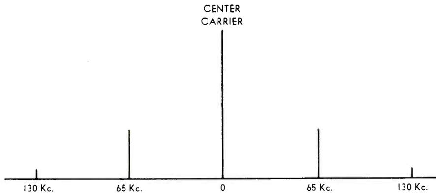
Figure 2—With 15 per cent modulation of a 65 Kc. supersonic tone (used for a subcarrier), the sidebands are positioned as above. The outer pair are very weak and insignificant.
