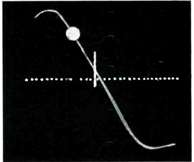
Fig. 5—The large white dot is placed to show the position of the main carrier when the receiver is tuned to one side. Only one of the 65 Kc. sidebands appears on the linear slope. The other one is lost. In this case, the sideband which appears on the slope will be detected as it deviates with modulation. The shorter the linear portion of the slope is, the more exaggerated will be the condition.
