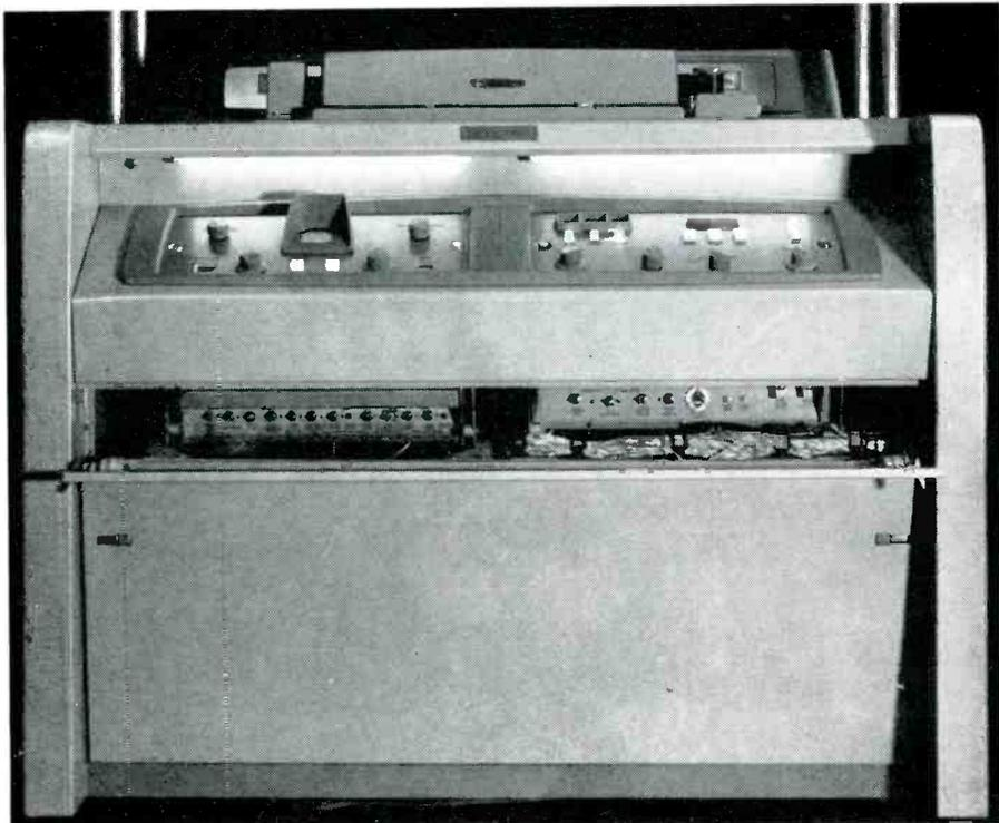
Front panels of VTR console dropped down, revealing easy accessibility of controls used by the operator in routine maintenance adjustments.
