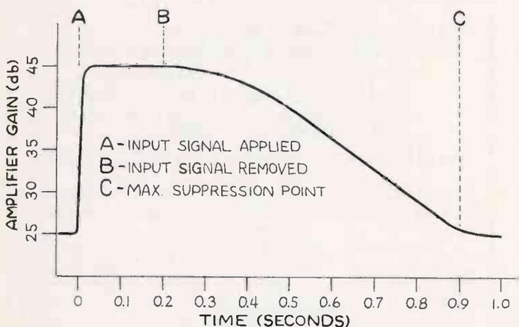
Figure 1. Gate Amplifier Gain Vs. Input Signal.
