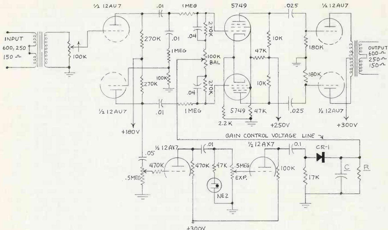
Figure 3. Simplified Schematic.
