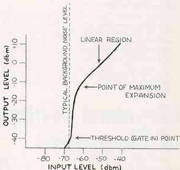
Figure 2. Amplitude Response.
