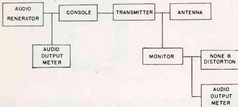
Figure 1. Block diagram of typical proof-of-performance equipment line-up.
