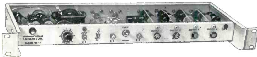
TDA2 VIDEO/PULSE DISTRIBUTION AMPLIFIER Output Gain: 4 or more
