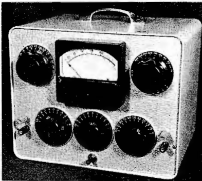
Fig. 1. The adjustable T-pad test set.
