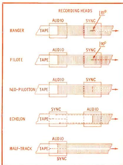
Fig. 1. Comparison of film-sync systems.
