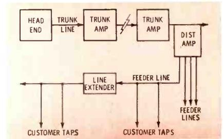
Fig. 4. Simplified system block diagram.
