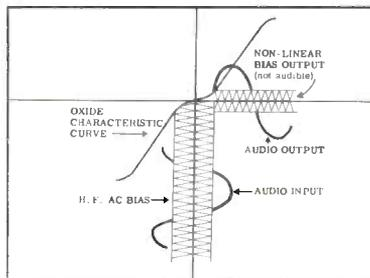
The amount of bias (that is the current in milliamperes) applied to the head is highly critical if top performance is to be achieved. Bias affects output, high and low frequency sensitivity, signal-to-noise ratio and distortion. This curve explains it.
