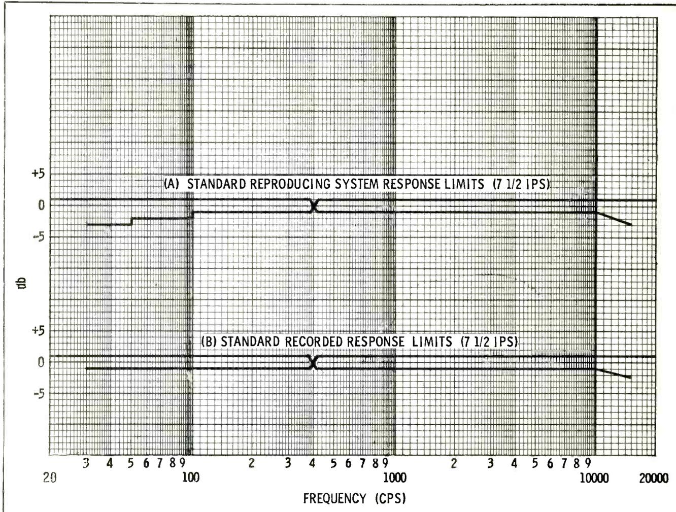
Fig. 3. These curves show the permissible limits between which the recording and reproducing responses may be allowed to vary.
