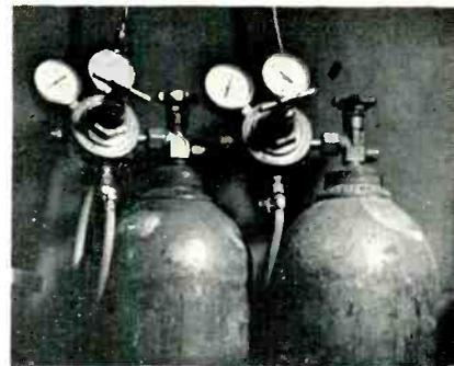
Fig. 3. Tank-mounted pressure gauges.
