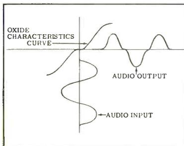
The slightly twisting curve at the upper left represents the oxide response. The lower curve is a pure, sine wave input. At the upper right we have the result of the response curve on the input . . . a mess.
