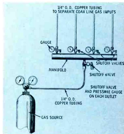
Fig. 4. Four sections fed by manifold.
