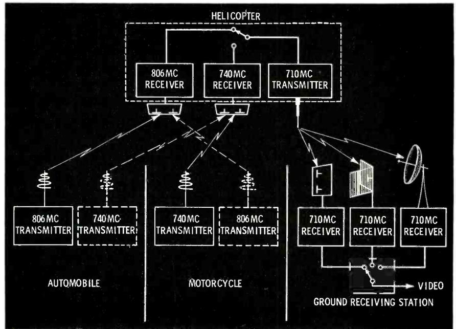
Fig. 4. Diagram illustrates the use of helicopter-borne equipment for TV relay.
