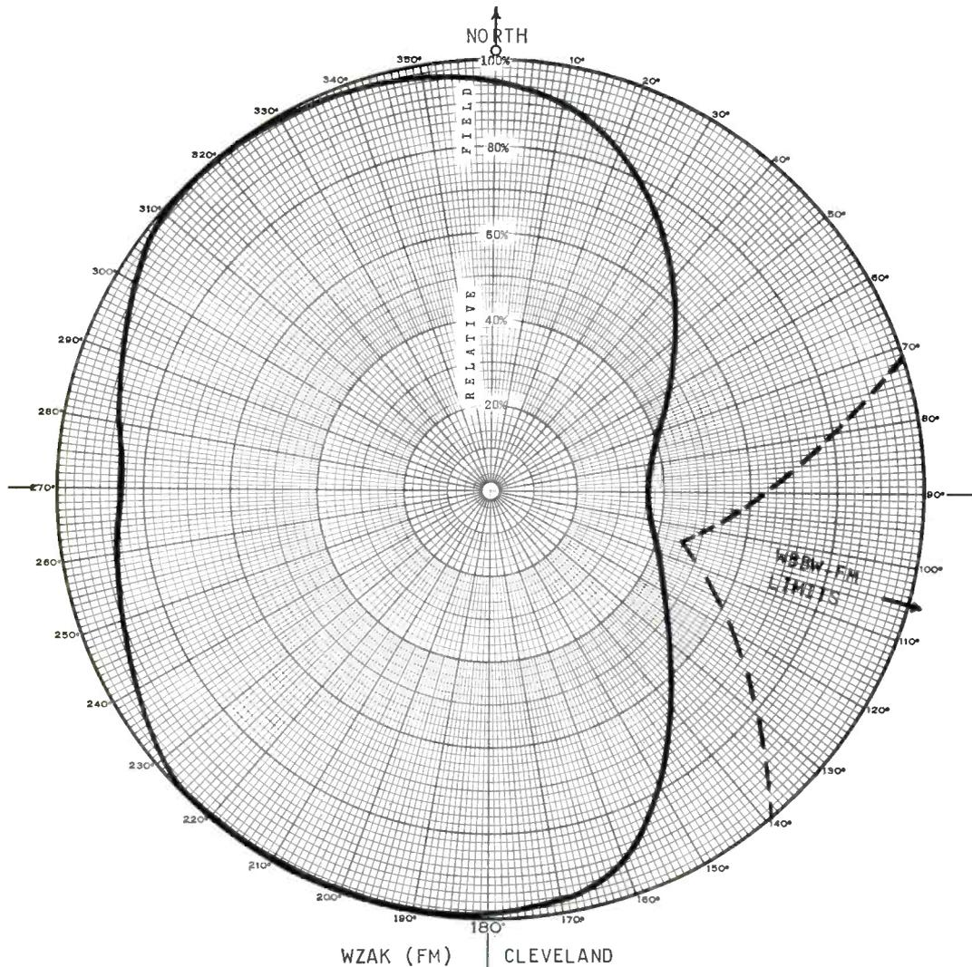
The FCC's 4th Order and Report now permits the use of directional FM transmitting antennas, to provide protection of short spaced stations. If you are now short spaced, you can, in most cases, increase your ERP in all directions except towards the short spaced station. Contact your consulting engineer for full details on how the new FCC Rules may help you increase your station's coverage.
