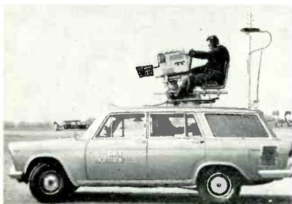
Fig. 1. Auto-top camera used in Italy.
