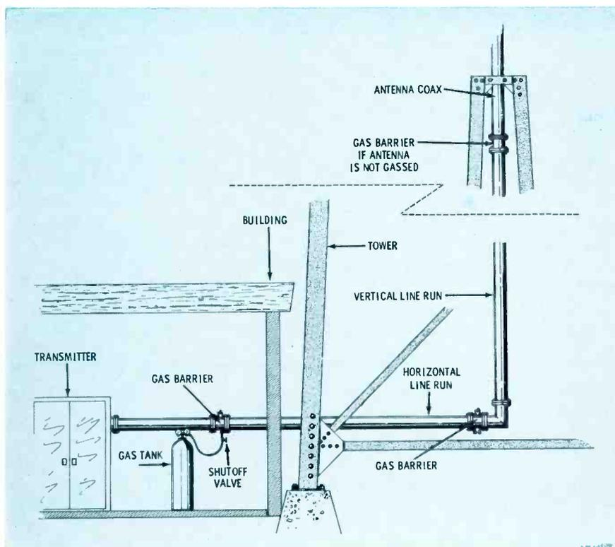
Fig. 1. Typical placement of gas barriers in a coaxial transmission-line installation.
