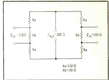
Fig. 3. Resistive pad for mixing & matching.
