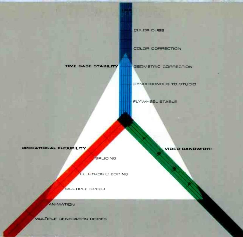
These parameters show the best that can be expected from present-day recorders. Note the limitations on bandwidth, time base stability and production flexibility.
