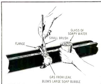
Fig. 5. Soap solution used to find leaks.
