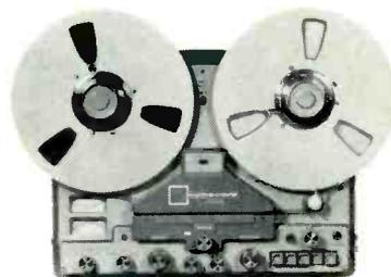
**MODEL 1048** The Model 1048 matches the Model 1028 in excellence of design and craftsmanship. Two speed ( $3\frac{3}{4}$  and  $7\frac{1}{2}$  ips) hysteresis synchronous motor, individual channel gain controls, half-track or quarter track stereo heads, four-digit counter and many features identical to the Model 1028.
