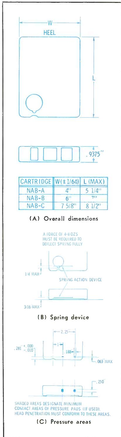
Fig. 1. Standard cartridge dimensions.
