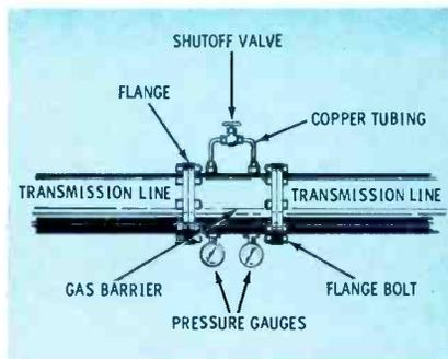
Fig. 2. Bypass and valve in gas barrier.
