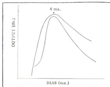
The steep curve represents low frequency sensitivity (measured in db.) at varying bias levels for many tapes. Note that you get good performance
