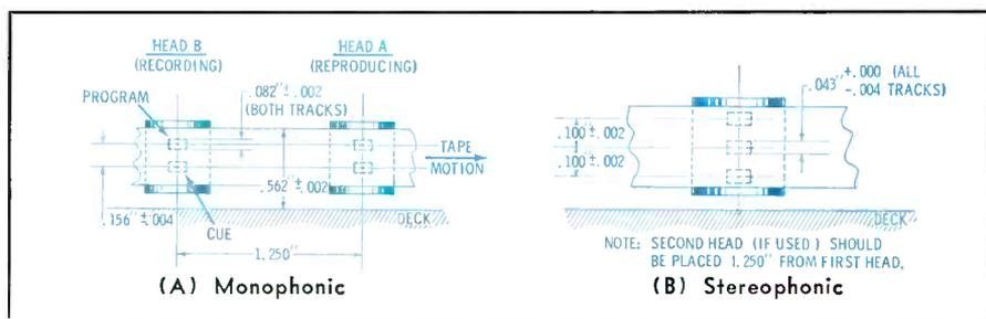
Fig. 2. Head and track configurations specified in the cartridge-tape standards.
